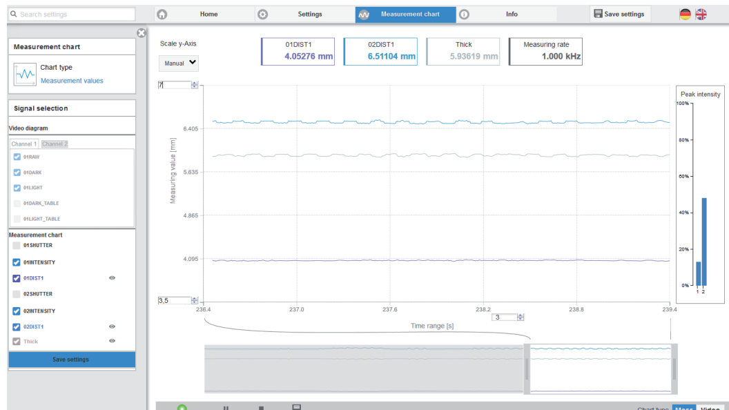
Fig. 78 Results from two-sided thickness measurement using two sensors
