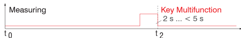
Fig. 63 Flow chart for resetting zeroing/mastering
