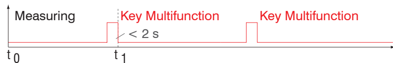
Fig. 62 Flow chart for zeroing, mastering (key Multifunction)
