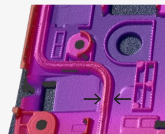
Inspection of height and thickness of adhesive beading on smartphone shells
